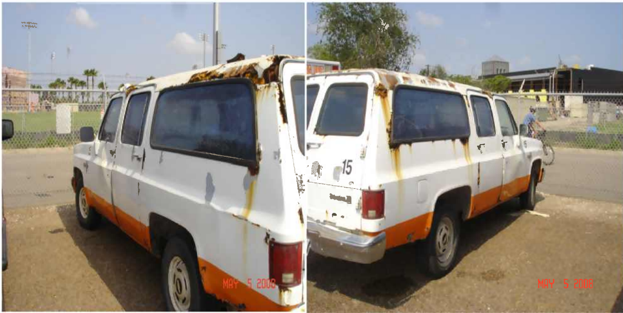
#15 - 1988 Suburban asset # 24412 – Vehicle body has heavy rust, leaks inside, age
