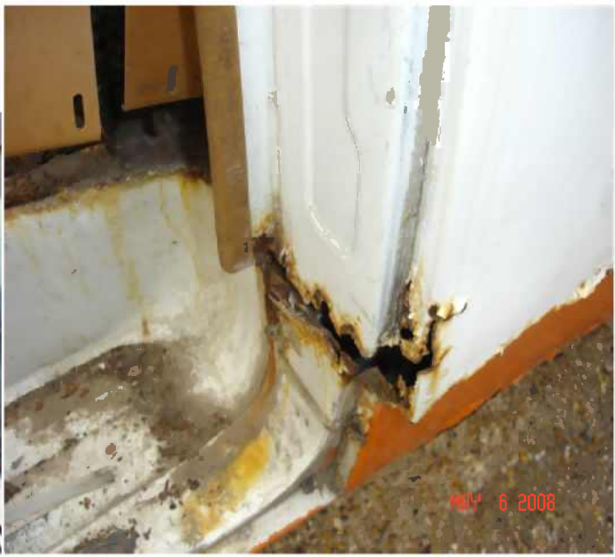
#7 - 1990 cargo van asset # 26444 – Vehicle body has heavy rust, leaks inside, age.
